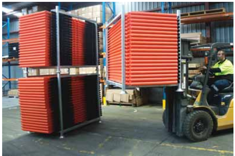
Q-fence stillages store 20 panels and stack easily with a forklift.
