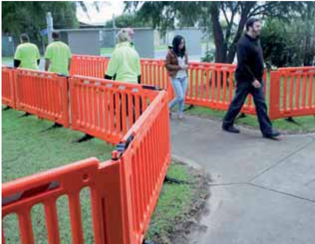
The lightweight, durable panels with recessed reflective strips are easily handled by one person.
