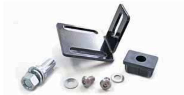
DF-APB Adjustable panel bracket kit Use in place of DF-SPB where side adjustment is required. Allows for up to 12mm of adjustment.
