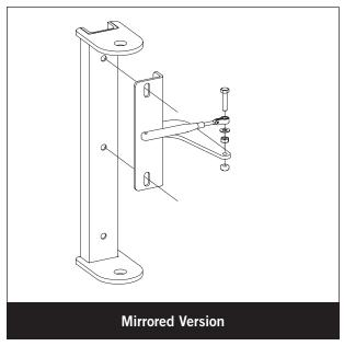
Gates can be set up to open left or right.
